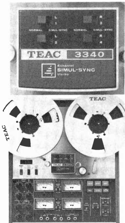
Fig. 7. The Teac 3340S multitrack deck. Inset shows Simul-Sync panel.
