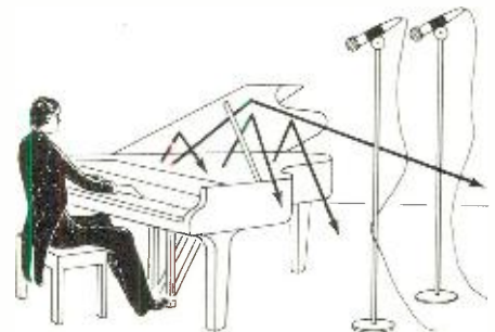
Fig. 3. This mike positioning for piano avoids pickup of direct reflections from bottom of lid.
