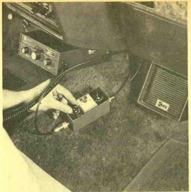
11 Testing with a standing-wave meter.
