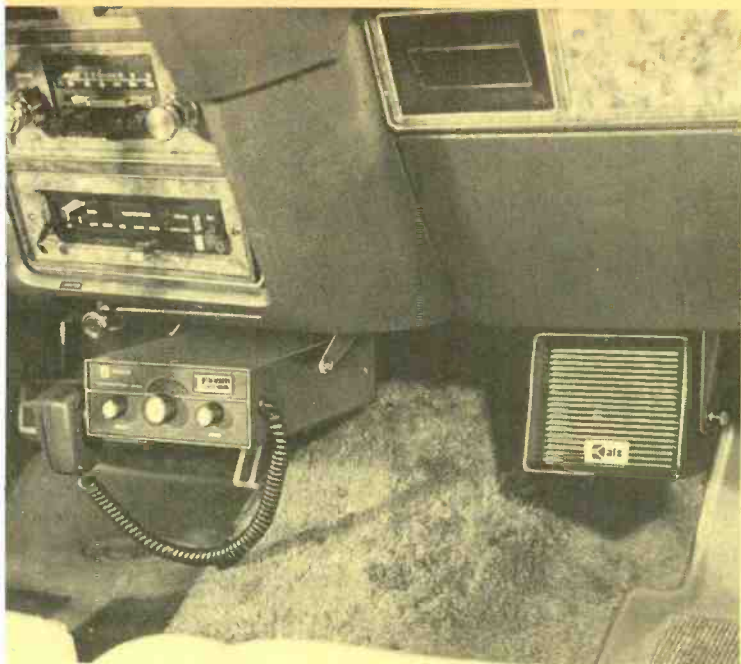
4 Transceiver and external speaker in place.
