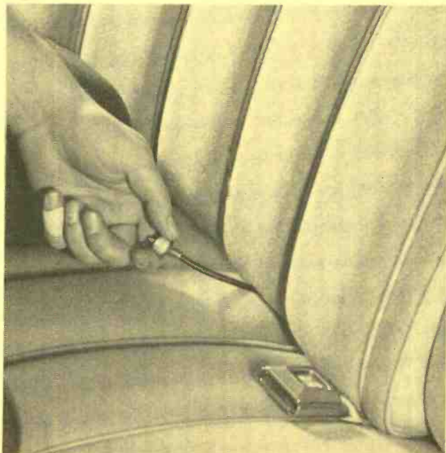
8 Pulling the cable from trunk into car.
