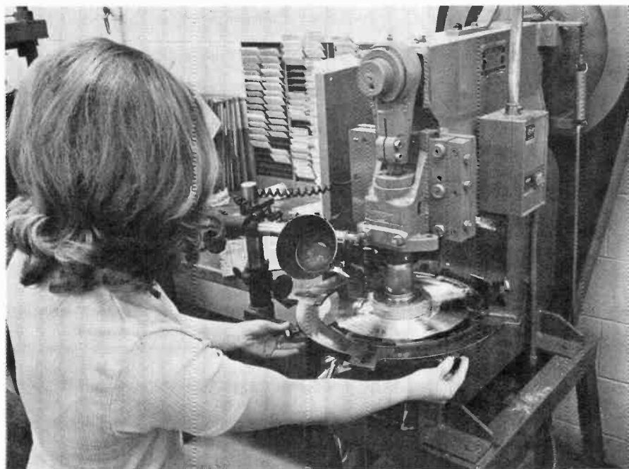
Fig. 6. Locating center hole for stamper involves spinning disc until groove pattern appears stationary.
