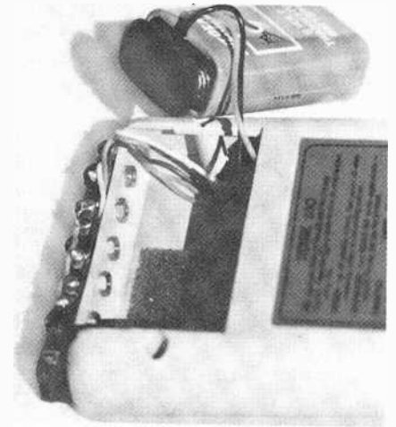
Arrange wires in battery well so they do not interfere.
