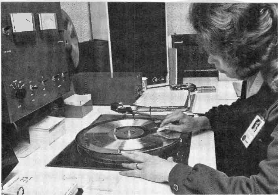
Fig. 5. Metal mother is played and imperfections are marked for later removal through "microsurgery."
