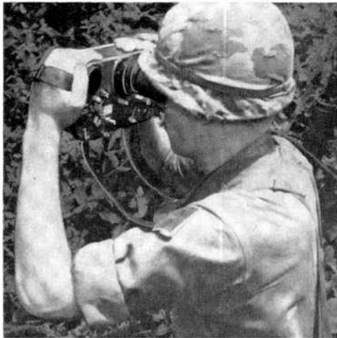
Handheld Thermoviewer detects objects by observing temperature differences.
