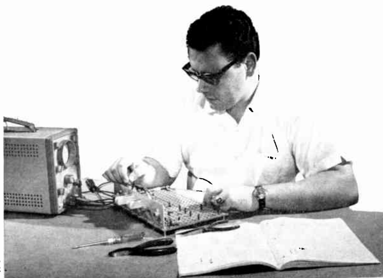
Performing transistor experiments on programmed breadboard — using oscilloscope
