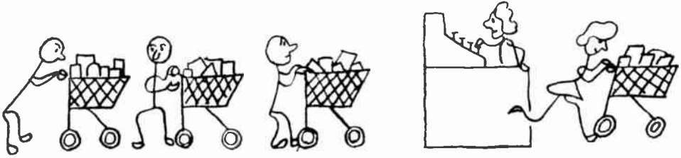
Fig. 3. Supermarket checkout counter can be used to explain "hole" flow in a transistor.
