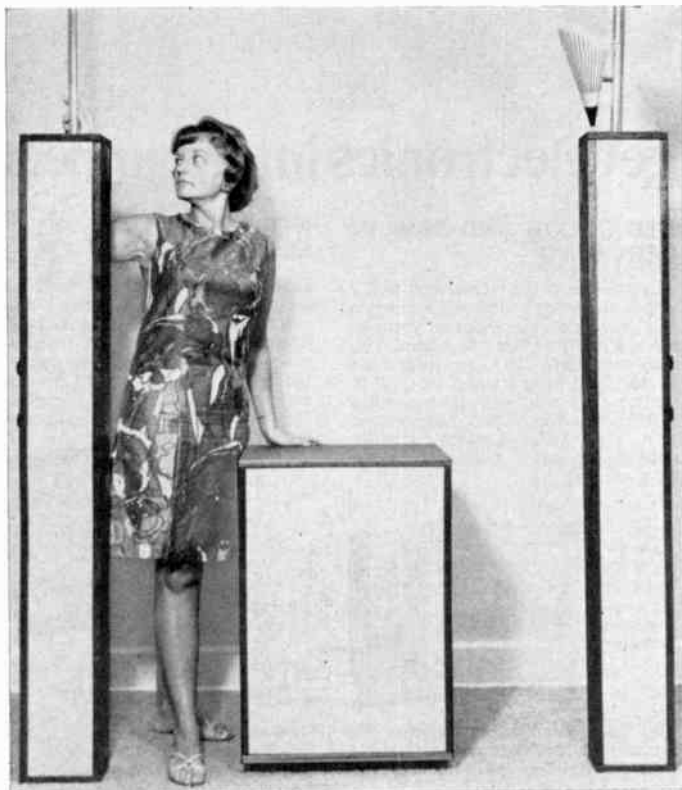
The mixed-signal woofer in the "Totem Poles For Stereo" project (January 1966) was located in the squat box shown in the center of the photo. The "totem poles" on each side contained the satellite speakers.
