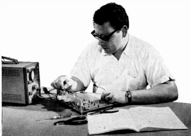
Performing transistor experiments on programmed breadboard—using oscilloscope
