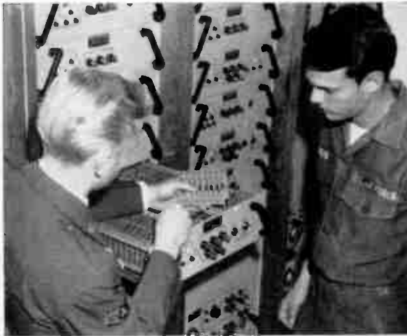
Instructor Sergeant Stephen R. DiStasio of Sacramento, CA, assists Airman Gerald W. Ralston of Grand Fork, ND, in running receiver sensitivity alignment of AN/GRC-169 Collins microwave transceiver (above) in Radio Relay Maintenance course.
