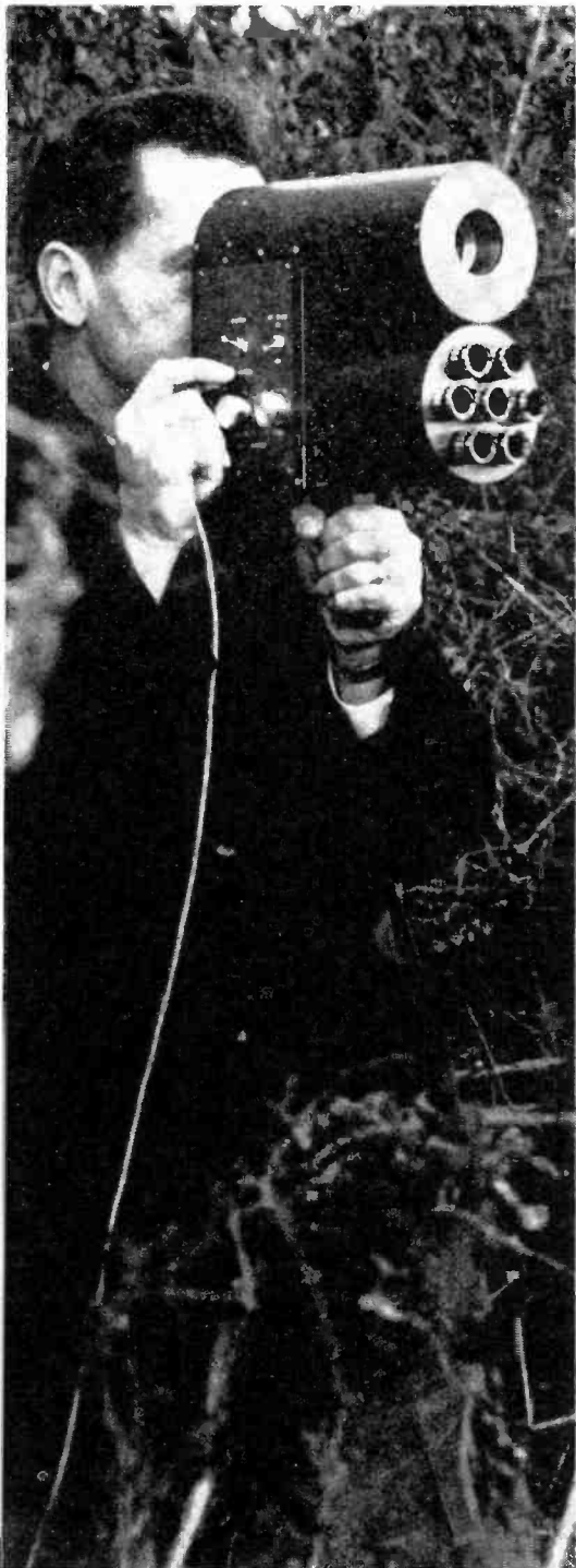
This detection system uses a gallium-arsenide pulsed laser and an image converter viewing tube to find targets up to 300 feet away in complete darkness. Developed by Laser Diode Laboratories.
