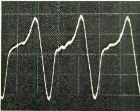
Fig. 7. Typical PPG displayed waveform. The trace shows fuzziness due to electrical noise pick-up.
