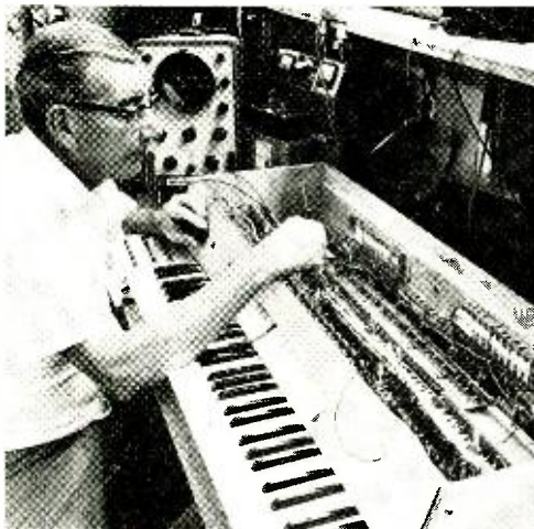
A 61-note keyboard, with 18 function and voicing stops, and a unique memory circuit are packed into the 36" x 20" x 6" Motorola electronic combo organ.
