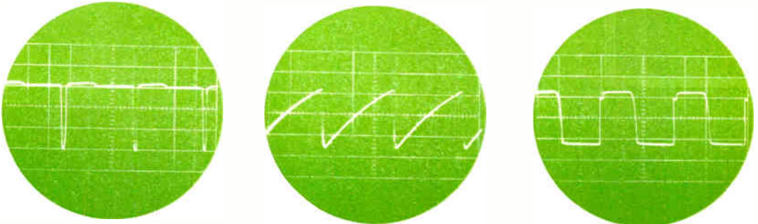
The pulse (left), sawtooth (center) and square wave (right) waveforms as seen on an oscilloscope. The little step on the leading edge of the square wave will vary dependent on the transistor used for Q2.
