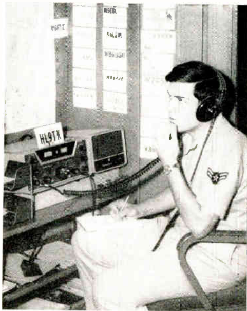
Airman Second Class John Ferrara initiated rescue operation at sea with his Hallicrafters SR-150 transceiver, running 100 watts PEP, and a Mosley V-3 Junior vertical whip antenna. (USAF Photo)
