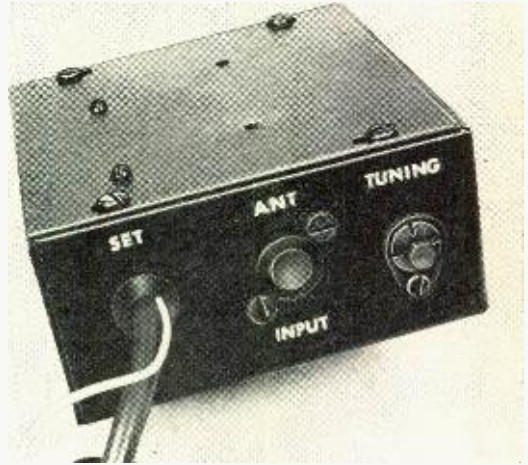
Fig. 3. Circuit must be built inside metal box to provide effective shield against r.f. interference that can be caused by ignition and other noises.
