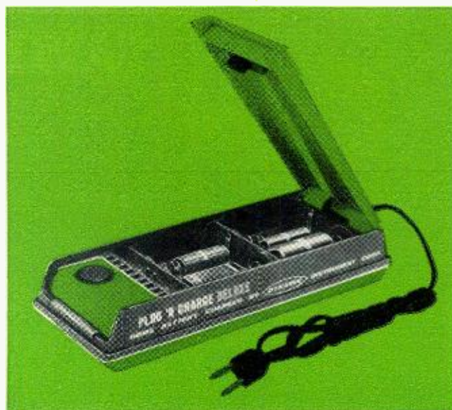
Fig. 3. This inexpensive, commercially available unit, with modification, was used to charge the batteries. An interlock similar to the type used on TV sets prevents the a.c. line voltage from getting at any of the exposed battery connections while the lid is up.
