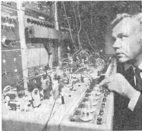
HOW TIME FLIES —A 24-hour day shrinks to only 14 seconds on this analog computer developed by Honeywell Inc. The computer electronically simulates temperature, humidity, wind, sunshine—even hills and trees—to help researchers like Lorne Nelson (above) design building control systems for the future. In 24 hours' actual time, the computer can give a building control system the equivalent of 17 years' use. "Function generators" electronically duplicate changing weather conditions; and other components simulate windows, construction, etc.
