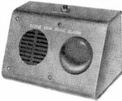
The author mounted his alarm in a sloping front cabinet, but there is no reason why other design housings won't work as well.
