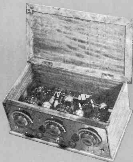
An early regenerative radio, a "blooper." Due to the large amount of r.f. they radiated, they could be heard in other receivers.
