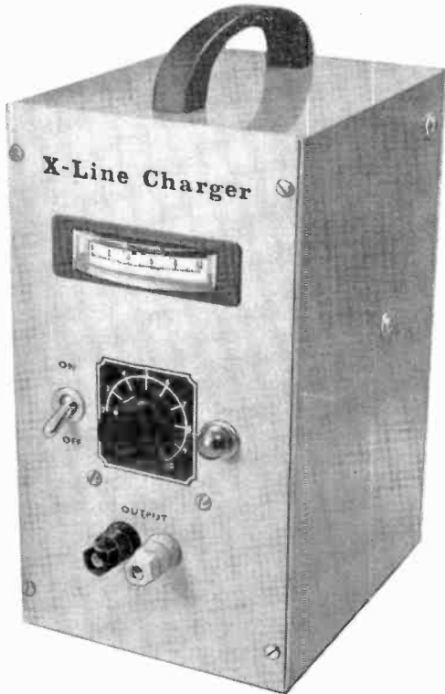
X-Line Charger has clean-cut appearance. Although not visible in photos, two screened \frac{3}{4} " holes are cut in the bottom and back panel for ventilation.
