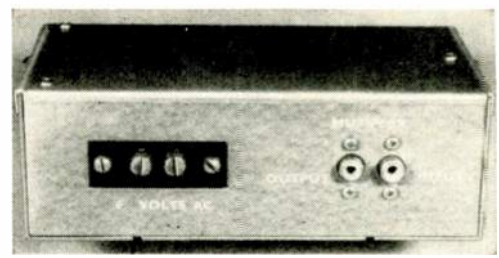
Fig. 2. In the self-contained unit, all connections are made on the rear panel. The name "Multiplex" refers to a function that no longer applies.
