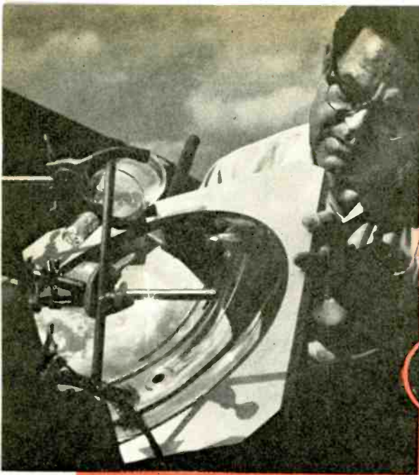
Sunlight pumping of a solid-state laser is a new development which may soon make it possible to put sun-powered lasers aboard satellites for communications, tracking, and geodetic measurements. This device, designed by RCA, uses a 12" hemispherical mirror to focus sun on calcium fluoride crystal rod.
