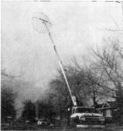
Mounted on a mobile tower truck, this parabolic dish is relaying a ham TV broadcast to Chicago from the QTH of W9EGQ, Gary, Ind. Herb participated in the dedication of W9DVJ via this TV remote pickup.
