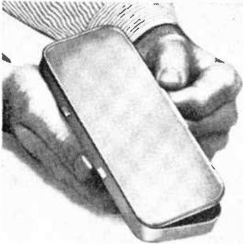
Fig. 7. First step in reassembly of mirror is to push pivot tabs on frame through matching slots in enclosure.
