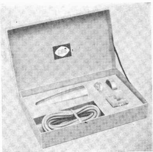
The eight pieces of the "Mark III" kit can be assembled in 20 minutes; assembled mike is semi-directional in position shown above, right, and omnidirectional when held vertically.
