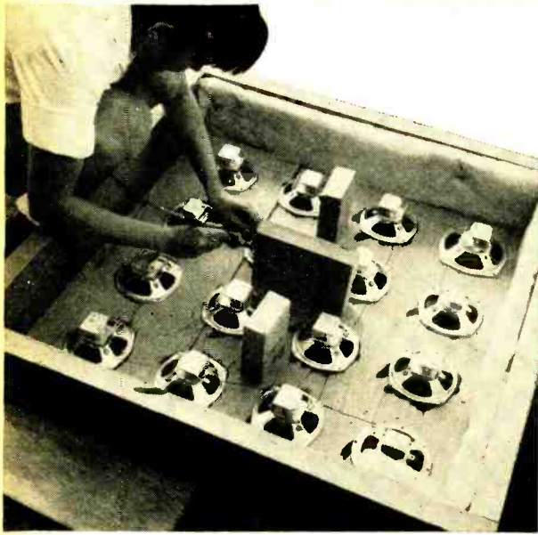
Connecting individual speakers is easy once you know the impedance you require. Simply use ordinary hookup wire and follow the appropriate schematic on page 57.
