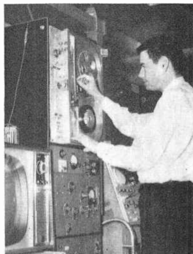
Dr. Glenn tests his prototype thermoplastic recorder. He estimates that he could halve its size by rebuilding it. Diagram of the TPR recorder is at left.
