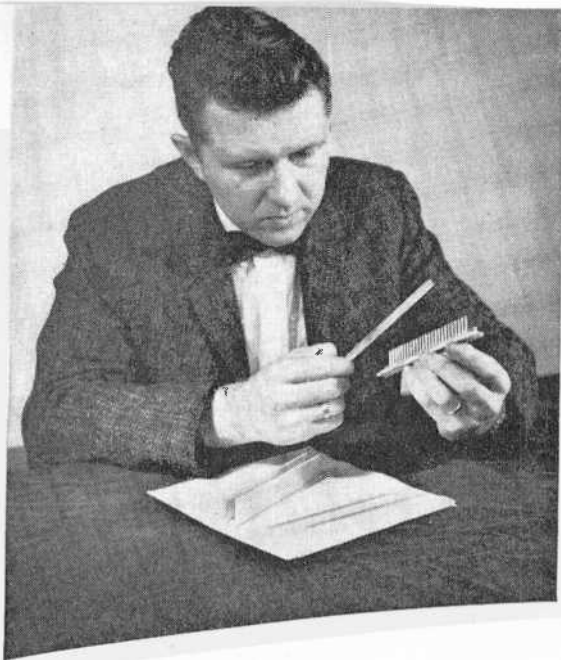
Disassembled maser is shown at left; scientist R. W. DeGrasse of Bell Laboratories holds in his right hand the strip of synthetic ruby which provides the amplification. The cutaway view of a maser (below) shows how the input signal weaves in and out of the row of pins next to the strip of ruby; each time the signal goes around a pin, additional energy is radiated, resulting in increased amplification.
