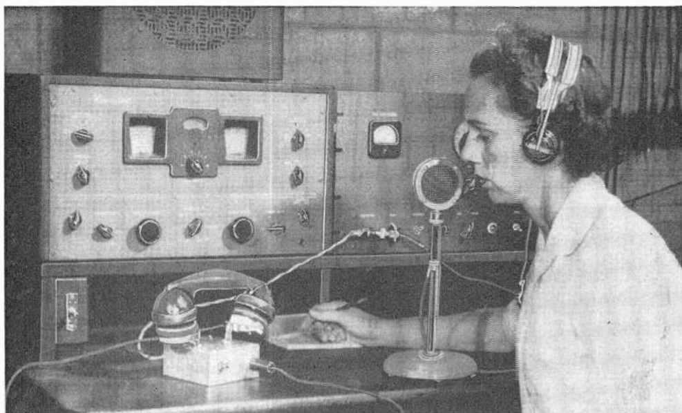
Typical radio amateur setup showing the telephone handset on top of the phone patch. The YL operator is monitoring the conversation between a contact on the air and a nearby friend on the telephone.
