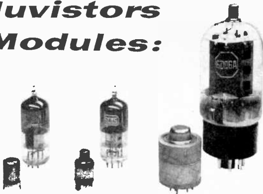
Three Nuvistors are shown beside their larger glass-tube counterparts. Left to right are developmental samples of a triode, tetrode, and beam power tube. Nuvistors outperform conventional types and make possible smaller, more efficient electronic instruments.
