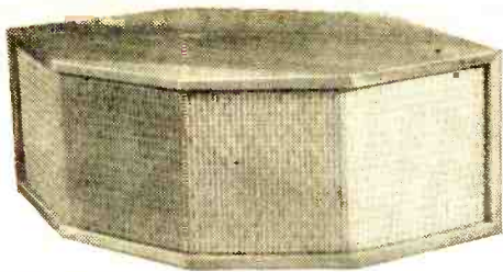
Four panels, at various angles for dispersal of highs, characterize the Janszen electrostatic tweeter, a push-pull unit handling 1000 cps and up.
