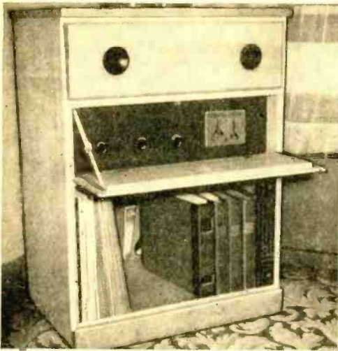
Front panel of second drawer hinges out to reveal preamplifier-equalizer and amplifier controls. Chassis are mounted behind panel.
