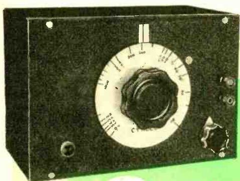
Fig. 1. Controls include frequency (center) and output (lower right)
