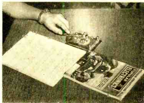
The best way to place the hand and fingers on a telegraph key is the way that feels most comfortable to the individual operator. The position shown in this picture is typical.
