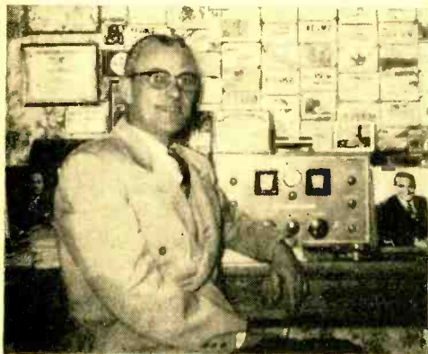
One of PE's steady reporters, Floyd Backus of Richmond, Va., uses an HQ140X receiver. His antenna is 102' long, 30' high. Since this photograph was taken, he has added an RME 22A preselector and a 24-hour clock.
