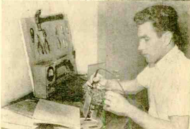
Final check on home-built set is made by student taking home-study course given by International Correspondence Schools, Scranton, Pa. Previously, the trainee had constructed the multi-tester he now uses for checking resistances. Signal generator at far right was also built.
