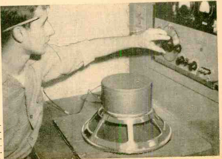
11 In the final stages of assembly, voice-coil leads are brought from spider to speaker cone. They are twisted into pigtails to prevent the damping of the cone as well as lead breakage.
