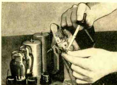
Cleaning the shaft of a potentiometer.
