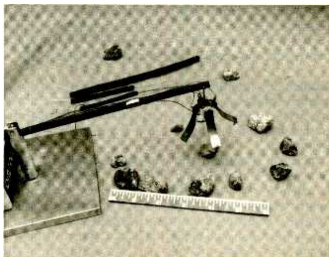
JPL's robotic arm was built mainly to demonstrate how EAP technology could be used to collect planetary samples on future space missions.
