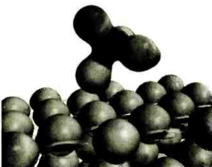
A computer image of arsenate ion sorbing on to an oxide surface. The image is generated using a form of quantum mechanical modeling called density function theory.
