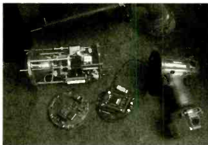
Researcher Gene Greneker and his team transformed the RADAR Flashlight from a bulky three-part prototype to a self-contained unit, weighing about seven pounds. (Photo by Gary Meek)
