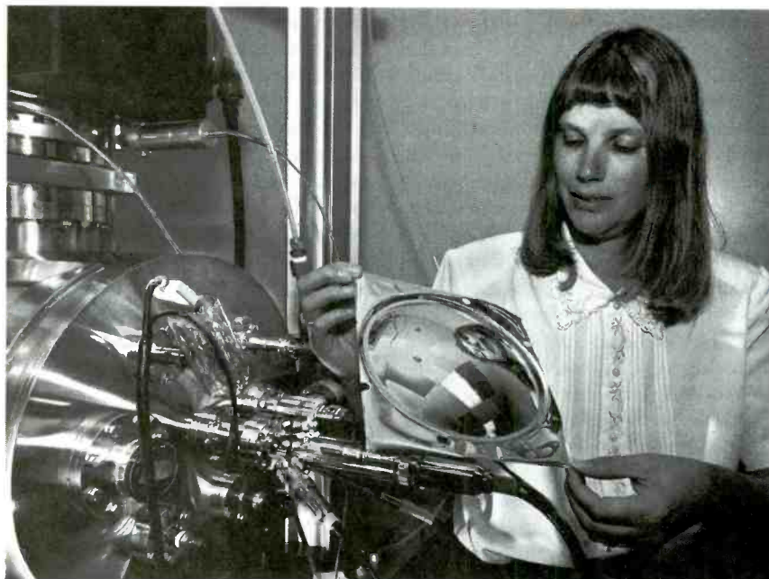
Sandia researcher Tammy Henson examines a new thin-film, ultralight piezoelectric material that may be the future of space telescopes and surveillance satellites. (Photo by Randy Montoya).
