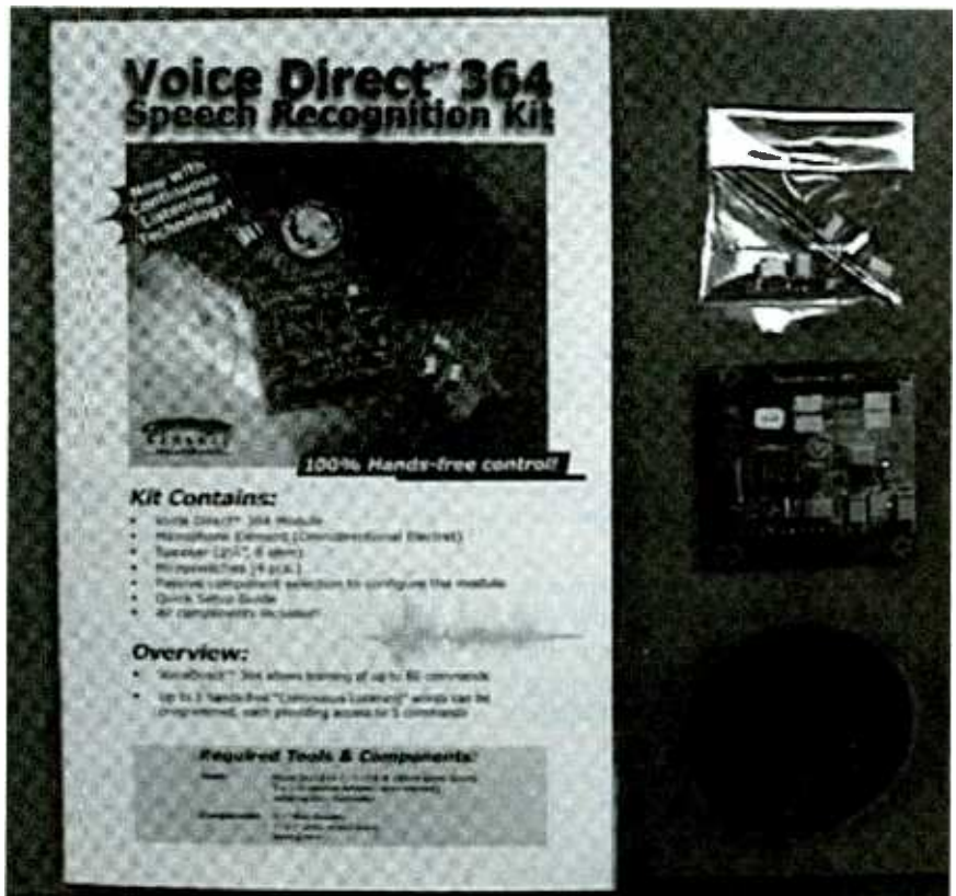
Fig. 1. The VoiceDirect 364 speech-recognition kit has a pre-built board that, with the included additional components, will have you issuing verbal orders to electronic equipment in no time.
