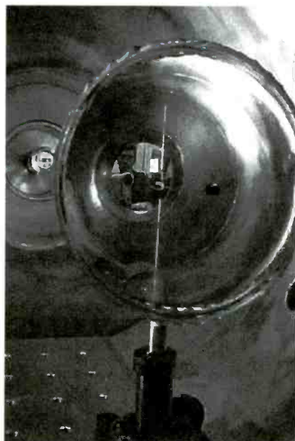
Shown here is the highly curved piezoelectric thin-film mirror inside a vacuum tube at the University of Kentucky.
