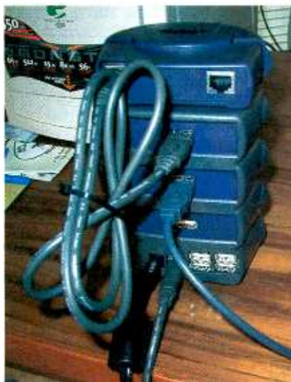
The Ethernet (or other add-on) module plugs into a USB port on the BusStation's rear panel.
