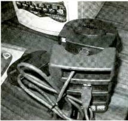
You can also pop out one of the USB ports and put an add-on module into the BusStation stack.
