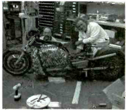
Designer and engineer Bill Dube (left) and another team member assemble a new pack of Bolder TMF cells into the KillaCycle.
