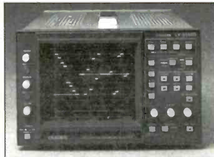
The first HDTV combination waveform monitor/vectorscope provides both serial digital (1.5GHz) and analog HDTV inputs.
