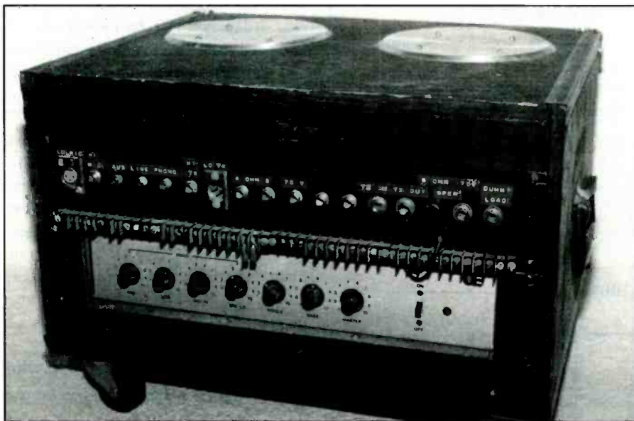
Figure 5. This portable audio test unit includes a public address amplifier, connectors, adapters, speakers, and other audio test equipment.
