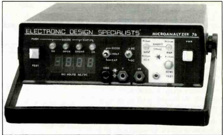
Figure 5. This unit contains several test devices that allow a service technician to perform a complete series of tests on a microwave oven.
