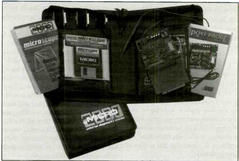
Figure 1. This diagnostic software kit features a software diagnostic application, a POST reader card, two technical manuals, a set of three wrap plugs, and a copy of the text, "Upgrading and Repairing PCs."
