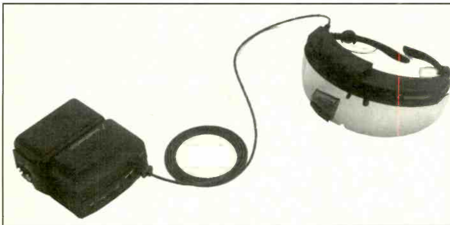
Figure 3. This pair of five-ounce portable eyeglasses with its attendant belt pack enables people to watch big screen TV wherever they go. With the glasses on, viewers see a big screen, color TV image that appears to float about 10 feet in front of them. The glasses also contain earphones that provide stereo-quality sound.
