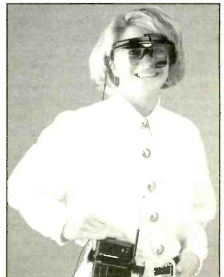
Figure 3. This pair of five-ounce portable eyeglasses with its attendant belt pack enables people to watch big screen TV wherever they go. With the glasses on, viewers see a big screen, color TV image that appears to float about 10 feet in front of them. The glasses also contain earphones that provide stereo-quality sound.
