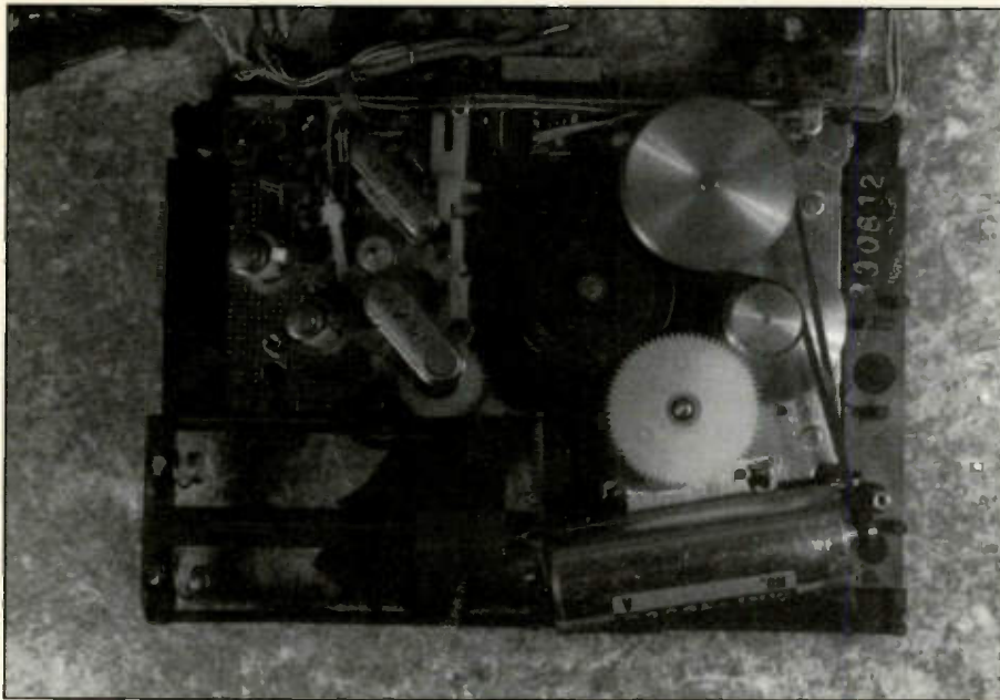
Figure 3. A transport with the circuit board removed. Note that the small cylindrical motor (lower right) is turned 90 degrees to the capstan and flywheel.
