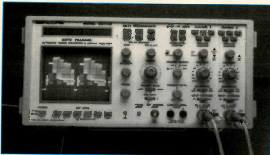
Figure 3. If you service video, make sure the scope on your bench offers complete video triggering and full measurement capabilities allowing you to measure the collector of the horizontal output transistor.
