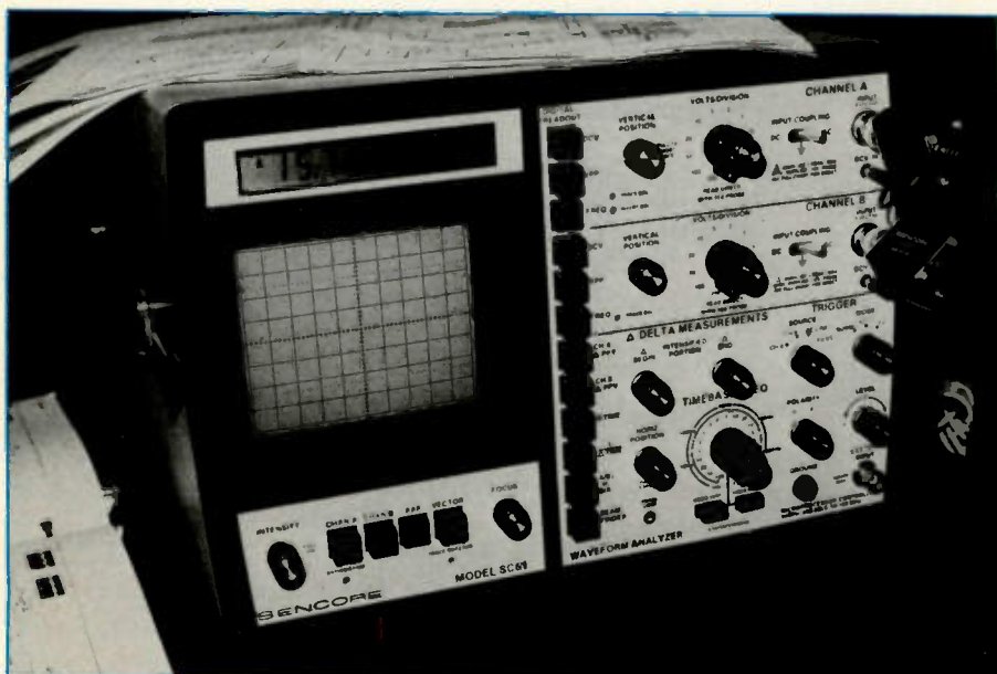
Figure 3. A waveform analyzer quickly locates defective waveforms and voltage measurements within the TV chassis.
