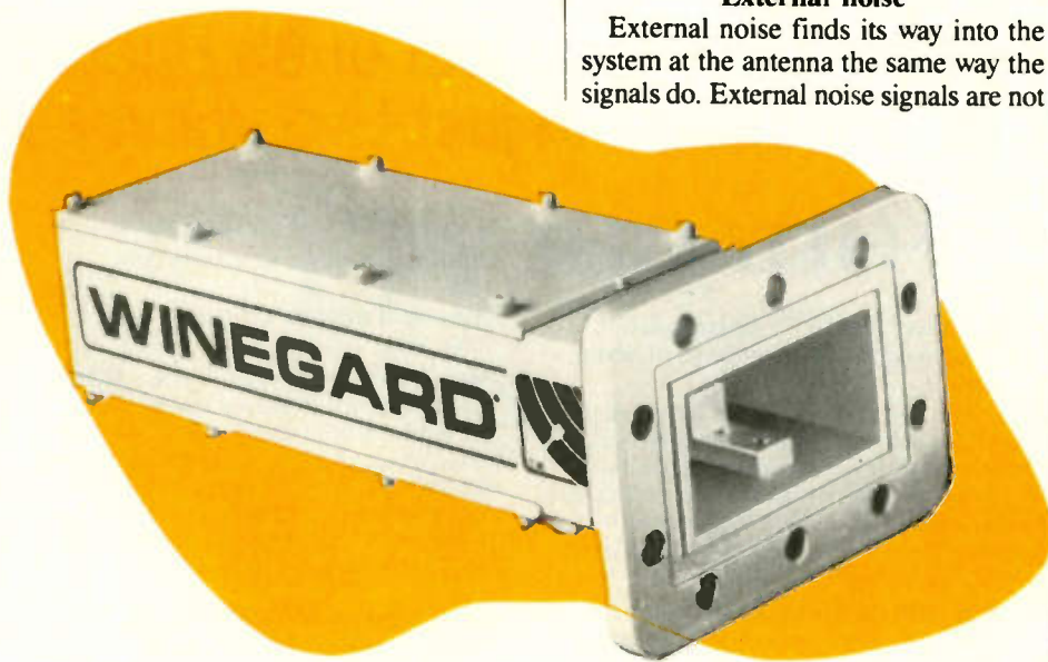
Figure 1. The LNA is a pre-amplifier that must be located directly at the antenna; otherwise, the received signal, which is extremely small, would be so attenuated and swamped by noise by the time it reached the TV set that it would be unusable. It is called a low-noise amplifier because it must contribute very little noise to the small-amplitude received signal that it amplifies, or it would contribute enough noise to make the signal unwatchable.
