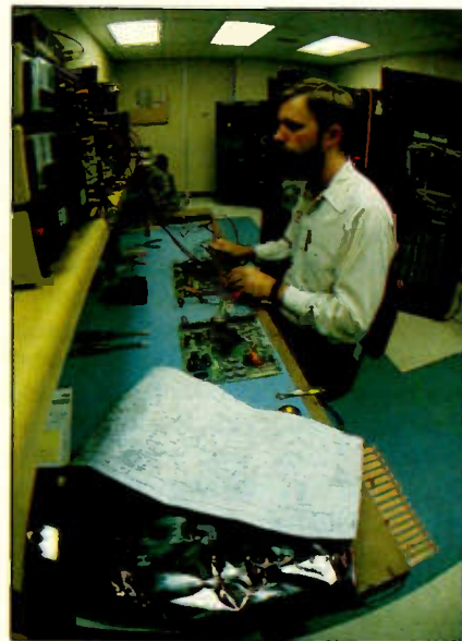
Circuit boards should only be tested or repaired at properly static-safeguarded workstations, which should include wrist straps, air ionizers, static-dissipative floor and table mats, and static-dissipative clothing.
