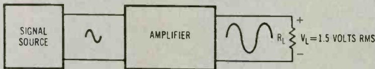
(B) The output amplifier is loaded with a resistor and the output voltage is measured.
