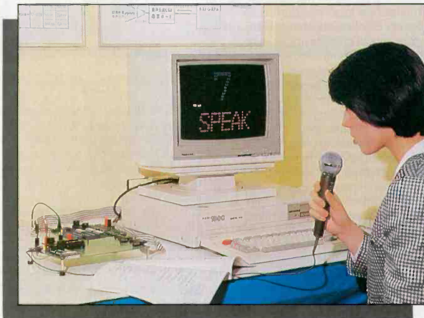
Trying out the speech recognition prototype LSIs installed in a Toshiba personal computer.
