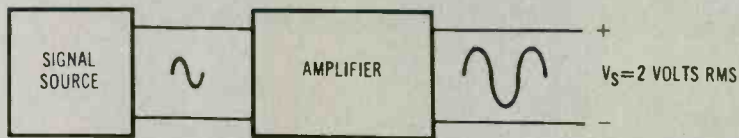
(A) A source is connected to the input of the amplifier to produce an ac voltage at the amplifier's output.
