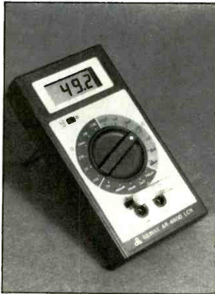
Model AR-460-D from American Reliance is a small meter for hand-held or bench use. It tests resistances, inductances and dissipations, also capacitances and dissipations.
