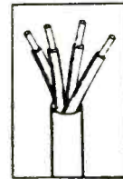
TELEPHONE STATION WIRE:
