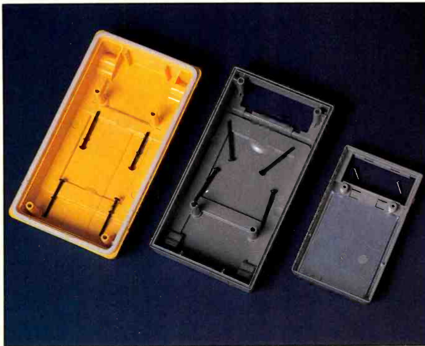
Shown left to right are the bottom cases of three DMMs. The major factor of mechanical protection is case design, including the number of internal ribs supporting the case, thickness of the material and number of screws holding the case together. For protection from contaminants such as water, a gasket is needed, as shown in white on the yellow heavy-duty meter.
