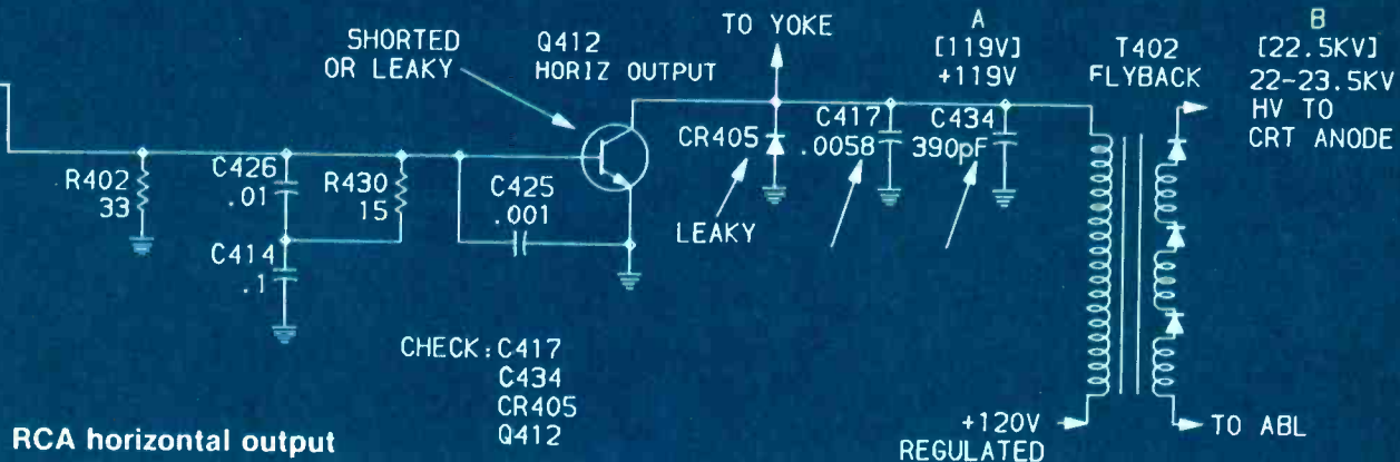
Figure 4. The horizontal-output stage in RCA CTC107 color receivers is not different in general from many other brands and models. However, many details are different. Arrows point to components most likely to cause overloads or excessive high voltage. Notice the flyback is the integrated type having HV diodes inside the HV windings.
