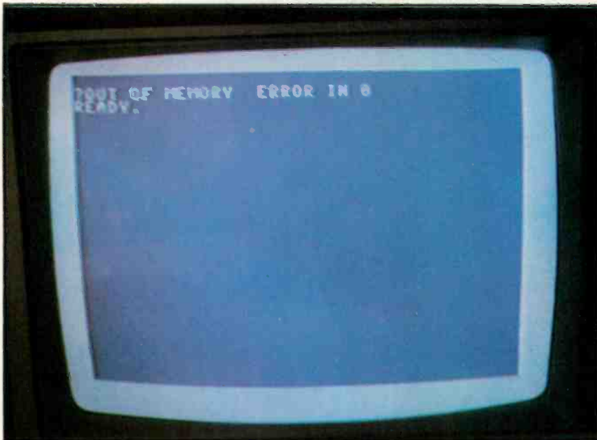
A number of programming errors will cause an OUT OF MEMORY ERROR message on the screen, but when you get this message at power-on you know that there's a defective RAM somewhere.
