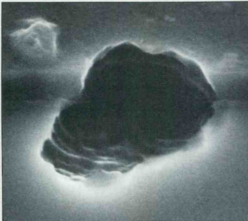
At 5,000 times magnification, the character of the damage can be observed. Some of the aluminum metallization has melted and can be seen along the bottom edge of the hole.
