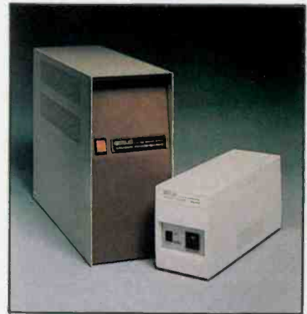
Standby power sources (SPS) provide clean, regulated ac power to critical loads when ac power fails or drops 15% below nominal. SPS units are available with outputs from 1,200VA down to 300VA.
