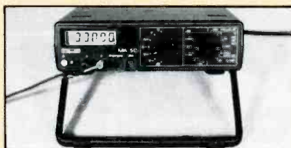
Figure 1. Model MA-5D from BBC-Metrawatt/Goerz is a high-accuracy 4- \frac{3}{4} digit DMM with \frac{1}{2} -inch high LCD digits in the readout giving a maximum count of 29999. All functions are selected by one knob, and the ranges are selected by a second knob. Only two test-lead jacks are used, except when 20A current is measured.
