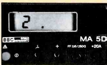
Figure 2. As shown, overrange activates the leading digit two and the decimal for the range. The display does not flash. Negative voltages and currents are identified by a minus sign at the left, but positive values or ac produce no polarity sign. Notice the German ground emblem above the negative probe jack.
