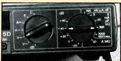
Seven functions can be selected by a knob near the front panel's center. Up to six ranges of the selected function can be selected by the knob at the panel's right.
