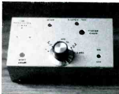
Drill all the holes in the cabinet prior to lettering and coating with a protective Krylon coating.
