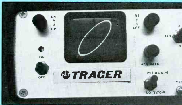
Figure 2. Certain values of inductances and capacitances produce oval waveshapes. Left, a 0.003 \mu F capacitor vs. the 10V/division sensitivity setting of the TR-1 created this oval shape and its angle. Right, an audio transformer caused the oval waveshape to tilt counterclockwise (opposite the capacitance tilt).
