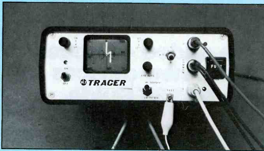
Figure 4. This waveform indicates a zener diode is across the test leads. The same waveform is obtained by connecting to the test jack on the panel.
